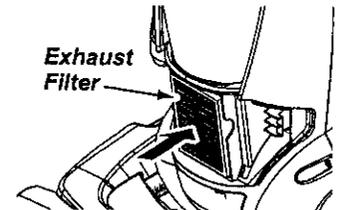
Replace the exhaust filter cover by placing tabs in slots and pushing in until cover snaps into place.
